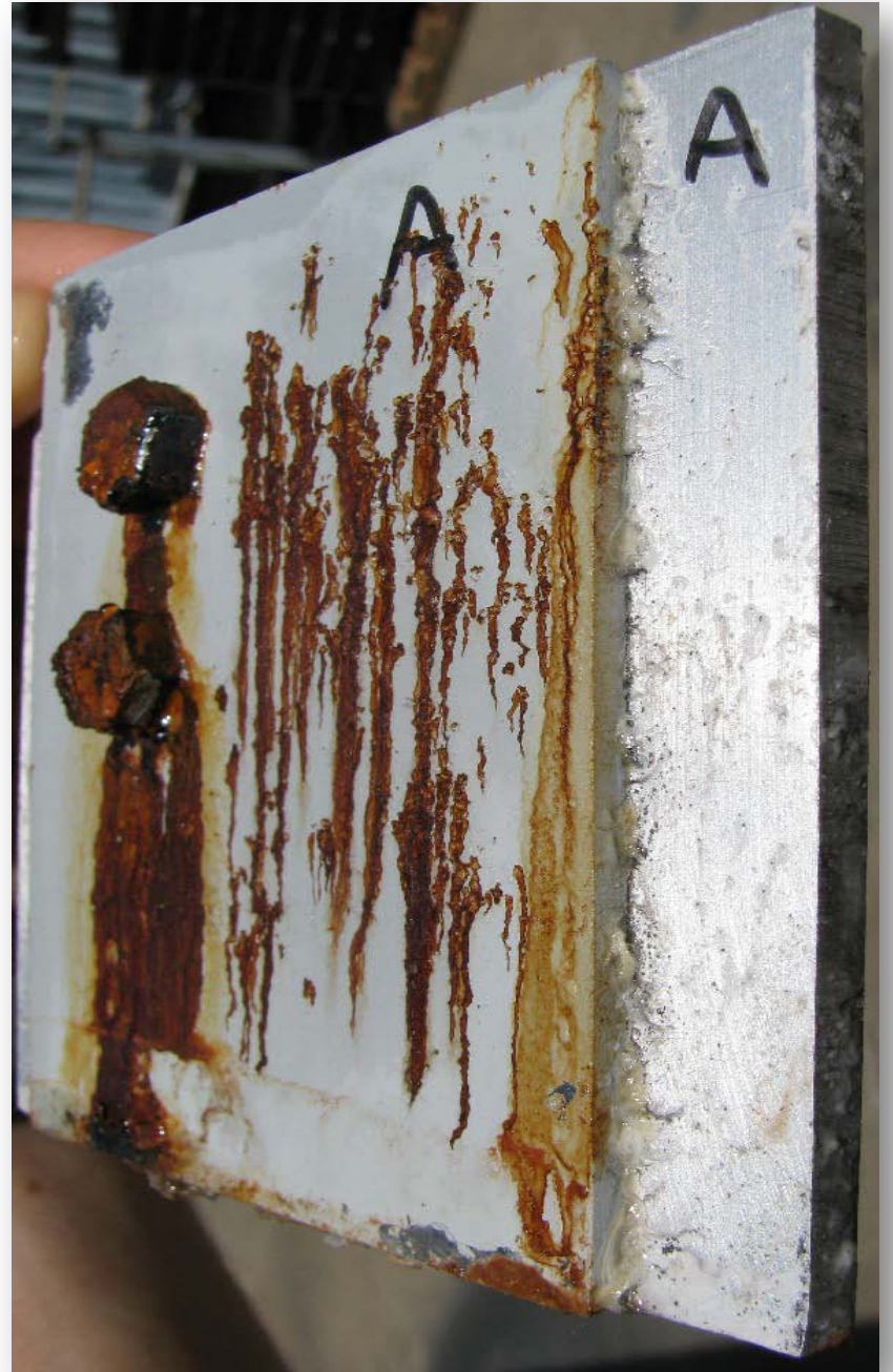
- Salt Spray Corrosion Test Results: 250 hours exposure in ASTM B117
